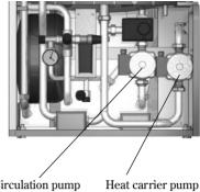
Circulation pump for the heating system (290 A/W) (290 A/W)
